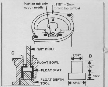
The other way to measure the float level is move the seat so it is .165 thous. from the top of the chamber to the top of the seat, figure C. There is a small tool you can use to set the proper distance of .165 thous., figure D. This tool is also available from our parts department.
